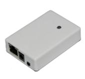
To control infrared equipment, Soline uses a universal remote control that can be controlled via the computer network. Such a remote control can control all the equipment that is in its field of vision or up to six different pieces of equipment if the module is «hidden» in a wardrobe. The user can control it with simple commands such as «Soline, I want to watch BBC» or «Soline, next channel».
