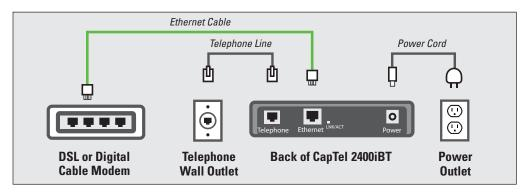
**Example 2:** If there is not an available Ethernet jack in your DSL or cable modem, you will need a router or switch that lets you connect more than one device to the Internet. Contact your Internet Service Provider to learn what router or switch will work with your modem. The router should support DHCP. Connect the router to your DSL/cable modem. Then connect the CapTel 2400iBT to the router or switch using the Ethernet cable.
