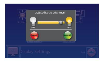
You can adjust the brightness of your CapTel 2400iBT display screen to make it easier to read in well-lit or dimly-lit environments.
