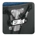
The control unit for the seat and backrest functions is on the back of the backrest. Easily accessible for the attendant.
