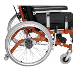
Seat height can be lowered -5 cm on the Bumblebee HD 500 model with alternative wheels 20" and 5" castors, enables the user to touch the floor with his or her feet.
