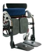
Legrest 90°, swing away, removable and angle adjustable between 90-130°. To be combined with castor adapters and 5" castors.
