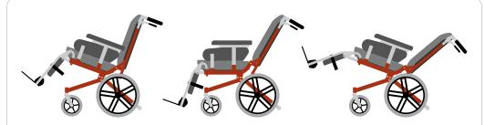
The seat unit can be tilted between 0° and +20° as standard. With an extended tipping bar the tilt can be increased to  $+30^{\circ}$ . Extended tipping protection must be used. The back can be tilted steplessly using a gas spring from 0° to 30° as standard. With an extended gas spring the back tilt can be increased to 50°. Extended tipping protection must be used.
