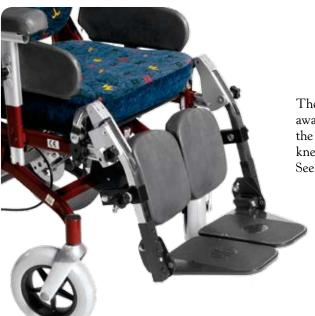
The Children's wheelchairs come as standard with swing away, removable and angle adjustable legrest. The angle of the legrest can be adjusted in steps from about 105° to 140° knee angle. Separate calf pads and footplates as standard. See accessories for more options.
