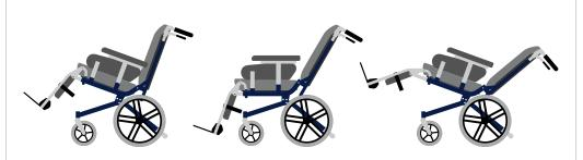
The seat unit can be tilted between  $0^{\circ}$  and  $+20^{\circ}$  as standard. The back can be tilted steplessly using a gas spring from  $-5^{\circ}$  to  $25^{\circ}$  as standard.
