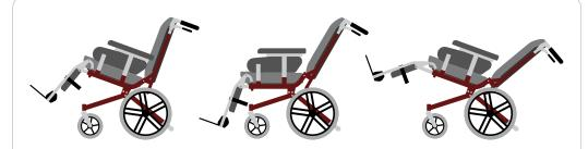
The seat unit can be tilted between  $0^{\circ}$  and  $+20^{\circ}$  as standard. With an extended tipping bar the tilt can be increased to  $+30^{\circ}$ . Extended tipping protection must be used. The back can be tilted steplessly using a gas spring from  $0^{\circ}$  to  $30^{\circ}$  as standard. With an extended gas spring the back tilt can be increased to  $50^{\circ}$ . Extended tipping protection must be used.
