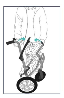
**3**. Place one hand at the top on the backrest bar and the other on the folding lever underneath the seat and by pressing it and bringing your hand together, close and fold the eFOLDi Powerchair.
