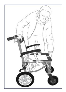
**1**. Once removed from the packaging place the wheelchair on a stable surface. Place one hand on the top of the backrest and the other hand on the latch bar underneath the seat, in the front part of the folded Powerchair. Finally push your two hands apart until the seat is open at 90° degrees and you hear a distinct "click" sound.
