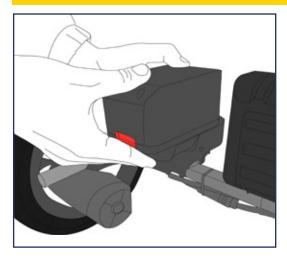
To remove the battery for charging, push the red button down, hold the battery on the outside, and release from the Powerchair. To put it back, slide the battery into the battery guide slot, push it until you hear a click, then the battery is inserted securely.
