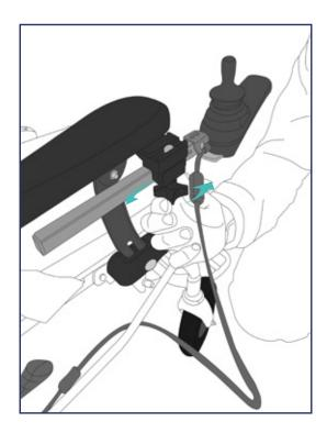
**3**. Finally slot the joystick arm inside the frame and push it, into a comfortable horizontal position, where it is easy for your hand to reach the joystick. Once you are happy with the horizontal position of the joystick arm, lock it by tightening the clamp.
