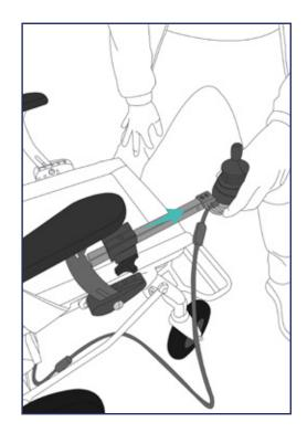
**1**. Loosen the tightening clamp, to release the joystick arm. Take out the joystick arm and place it on the Powerchair seat.
