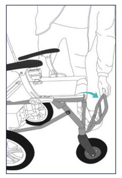
**2**. Unfold the footrest, from a vertical position to a 90° degrees horizontal position.
