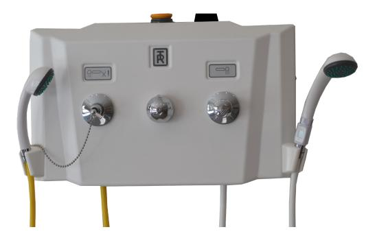
TR 2810 is a shower panel with a built in thermostatic mixing valve and separate on/off valves for the shower system and the cleaning system. The cleaning system runs on cold water to minimize inhalation when cleaning equipment, the panel has a built in bottle for cleaning detergent. TR 2810 is now available with a mechanical lock for cleaning detergent bottle (option).
