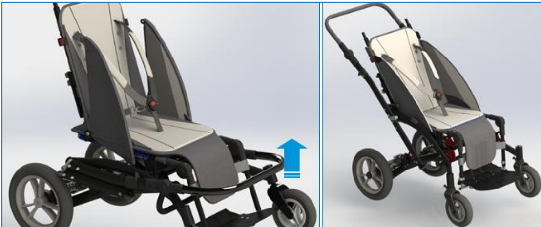
Fig. 6 Unfolding the buggy's frame
