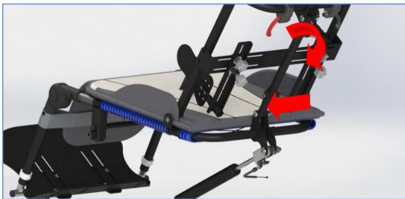
Fig. 33 Chest support width and height adjustment
