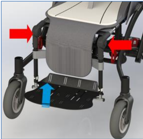
Fig. 36 Footrest supports angle adjustment
