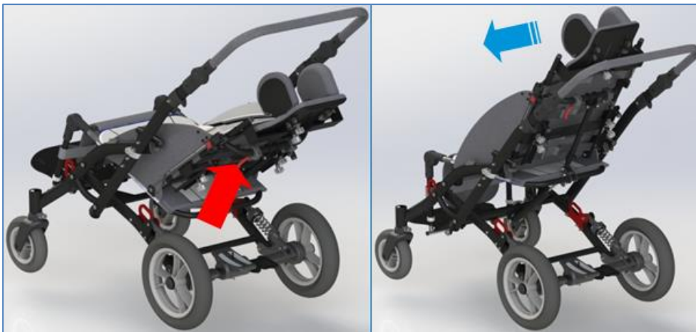
Fig. 17 Adjusting the angle of the seat
