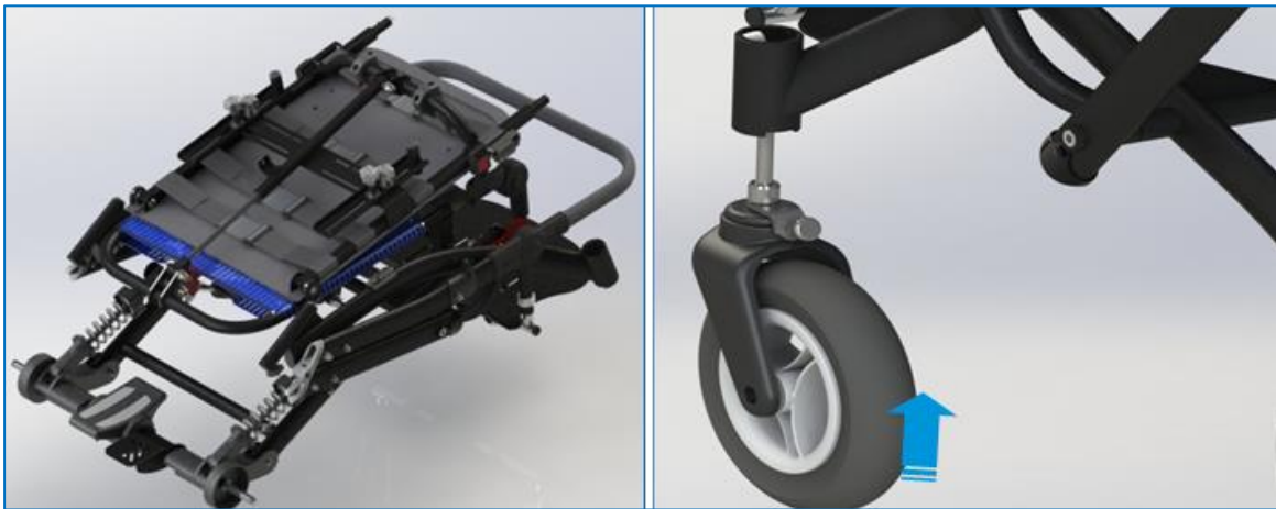
Fig. 2 Stroller frame, along with the seat
