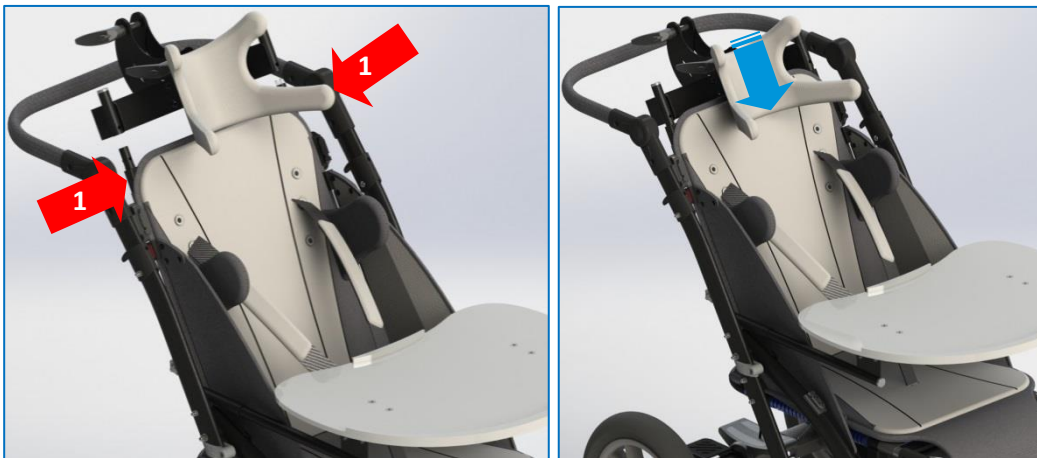
Fig. 9 Mounting the horned headrest
