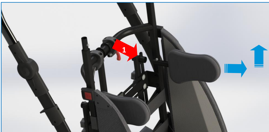
Fig. 18 Chest supports dismantling
